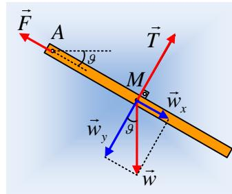
$$\Sigma \vec{F} = 0 \rightarrow \Sigma F_x = 0 \quad (1) \text{ and } \Sigma F_y = 0 \quad (2)$$
